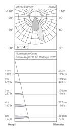
1466 - 1664lm 20W 77 - 86lm/W 500mA >83% 2700K - 5700K 3SDCM L80/B10 (>50,000hrs@Ta-30Deg C) Assymetric WW+DL <19 >90
