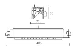
Cut-Out: 396 x 60mm \*All Dimensions are in mm.
