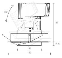
Cut-Out: Ø145mm \*All Dimensions are in mm.
