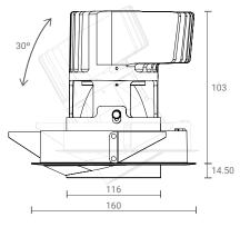
Cut-Out: Ø145mm \*All Dimensions are in mm.
